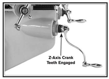
Figure 9. Z-axis crank installed.
